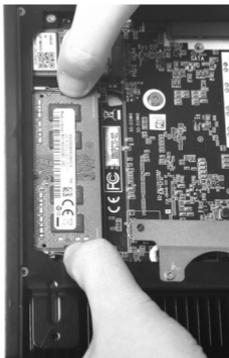
2. Remove the memory module from the slot at a 45-degree angle.
