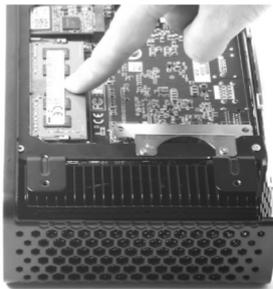
Note: This ZOTAC ZBOX nano accommodates two DDR5 SO-DIMM memory modules. You must install at least one module for the system to function. Windows models include memory pre-installed.
