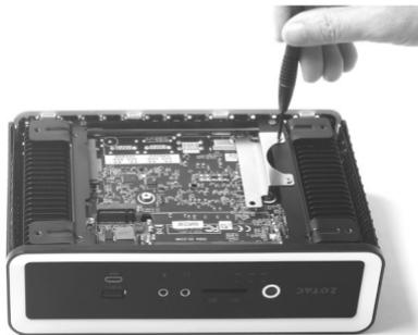
2. Install the SSD bracket to a 2.5-inch SATA SSD with 2 screws.
