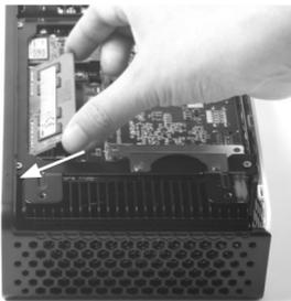
2. Gently press down on the memory module until it locks into place by the arms of the memory slot.
