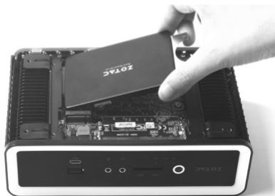
4. Reinstall the screws of the SSD bracket.
