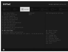
Change the status of Enable VMD controller and Enable VMD Global Mapping to Enabled.
