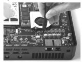
2. Insert an Optane memory module into the slot at a 45 degree angle.
