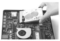
4. Secure the installed drive with a thumb screw.
