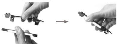
3. Insert the storage drive into the slot at a 45 degree angle and gently slide into the connector.
