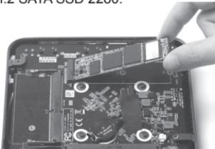
3. Attach the screw to the M.2 SATA SSD module as shown below.
