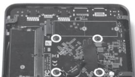
2. Insert an M.2 SATA SSD module into the slot at a 45 degree angle.
