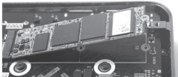
4. Gently press down on the M.2 SATA SSD module, and install the screw on board.
