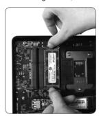
2. Remove the memory module from the slot at a 45-degree angle.
