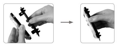
3. Insert the hard drive into the slot at a 45 degree angle and gently slide into the connector.
