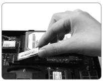
2. Gently press down on the M.2 SSD module, and install the screw.
