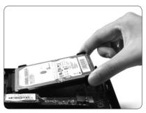
4. Secure the installed drive with a thumb screw.
