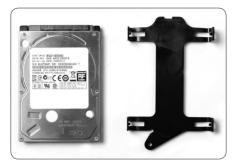
2. Install the hard drive to the hard drive bracket.
