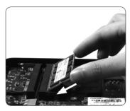
Gently press down on the memory module until it locks into place by the arms of the memory slot.
