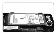
\*1 TB 2.5-inch SATA hard drive is pre-installed in Plus and Windows version.
