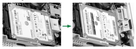
3. Gently remove the hard disk from the socket, close and screw the lid.
