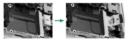
3. Insert the hard disk into the socket at a 45 degree angle.
