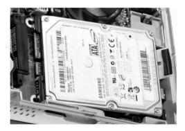
4. Gently press down on the hard disk until it is seated, shut and screw the lid.
