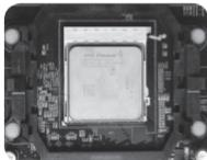
**Note:** Do not use excessive force to install a CPU. If the CPU doesn't easily fit into the socket, check the orientation of the CPU and realign the CPU until it fits with ease. Using excessive force may cause damage to the pins on the motherboard or CPU and void warranties.
