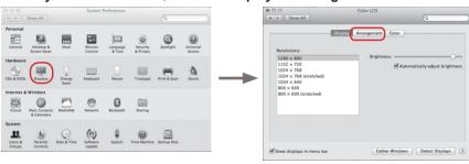
7. Now you can enable ZOTAC USB3DOCK HDMI monitor on the window below. ZOTAC USB3DOCK supports extend mode and mirror mode.
