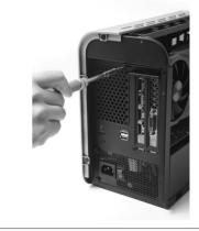
9. Install the cover with the three screws.
