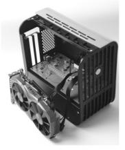
6. Insert the add-on card into the PCI-e slot.
