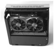
7. Install the screws to secure the add-on card.
