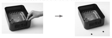
2. Gently lift up and remove the frame bracket.
