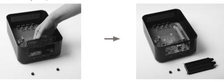
3. Press the lever of riser card and remove the riser card from the PCle slot.
