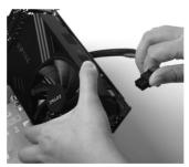
8. Insert the add-on card with frame bracket back into the box and slide the Riser card into the PCI-e slot.
