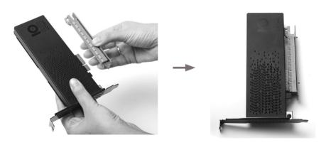
5. Remove the lower screw and remove the lower single-slot bracket.
