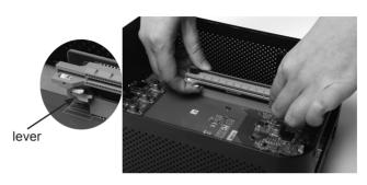
4. Install the riser card to your card (taking PCIe SSD as an example).
