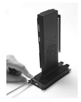
8. Insert the frame bracket with single-slot card into the Box, and press the riser card into the PCIe slot.
