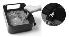
7. Connect the other end of the 6-pin power cable to the add-on card.
