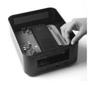
10. Reinstall the cover and the rear thumb screws.
