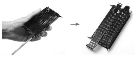
6. Install the single-slot card to the frame bracket as shown below.
