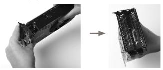
4. Tighten and secure the Graphics card to the bracket with the screws provided.
